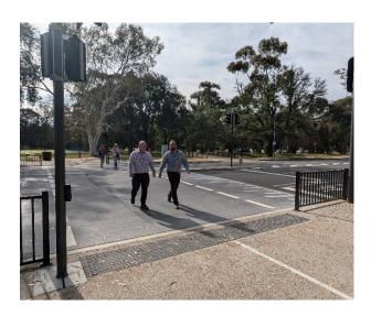
Bicycle Pedestrian Actuated Crossing (BPAC) with a raised safety platform on Hutt Road. This is an example of a primary Safe System aligned crossing outcome.
